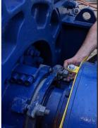
Figure 3: Large pump with **DualPac 2212** and **Live Loading** being installed.
