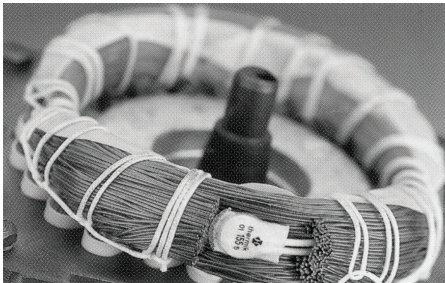
Thermal switch incorporated in windings
