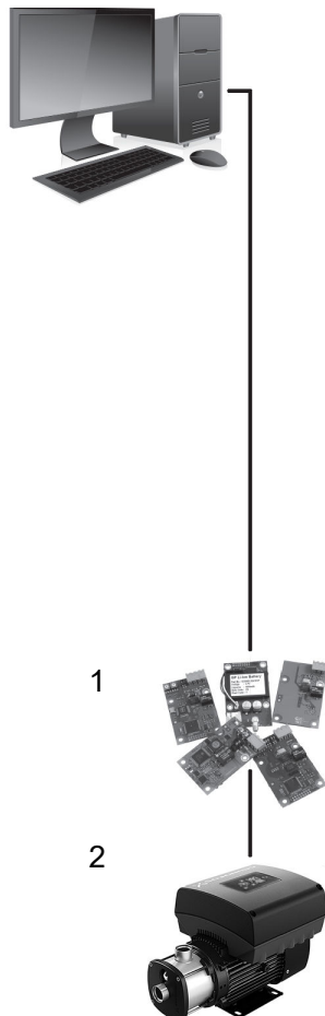
Communication via a central building management system
