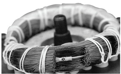
PTC sensor incorporated in windings
