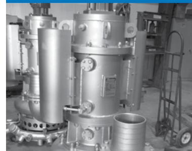
**The Original Agitation team - Toyo Agitator & Jet ring** - for applications where solids are especially difficult to pump, Toyo offers the option of a special high pressure jet ring. The jet ring combined with the original Toyo agitator have proven to be a truly effective 'agitation team'.
