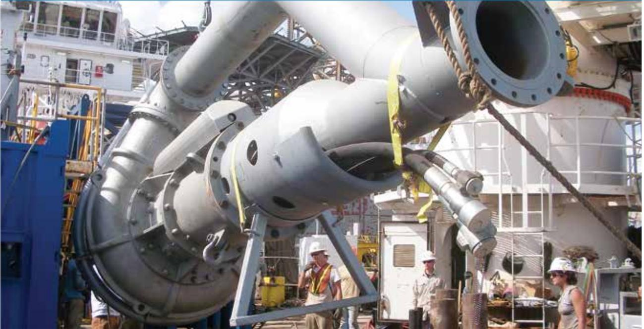
The **Toyo submersible DP series** and its hydraulically driven cousin the **TO series** were specifically designed to pick up and transport abrasive materials with the least amount of water.
